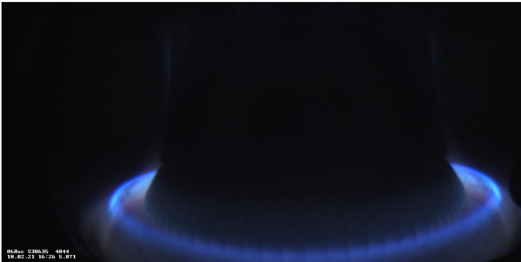
Figure 2.12: Camera image in the visible range of an X-point radiator plasma close to the L-H transition. A large fraction of power is radiated as line emission toroidally along the X-point due to the presence of nitrogen giving rise to the ring-like radiation structure. The divertor is detached in this situation. The usually visible D-alpha line radiation at the inner heat shield and in the outboard SOL does not appear due to very low temperatures in the SOL .
